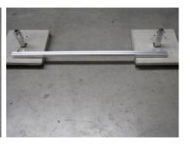
Insert the stand rails 300 mm (toe side) and 470 mm (manifold side) with the 5° cut in direction of the toe bar into the premounted profile angles of the longitudinal rails and fix them. Then insert the stand rails with the 45° cut into the basic plate and adjust the height (toe bar - bottom longitudinal rail min. 300 mm, manifold side – bottom longitudinal rail min. 470 mm). Please take into consideration that an inclination of 5° (from manifold side towards toe side) is necessary.
