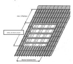
The bearing surface for the collector arrays must be adequately stable. If the gaps between the roof laths or rafters are very large, additional roof laths should be installed.
