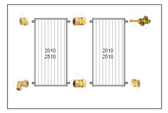
Fig. 1: Connection of collectors, vertical
