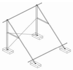
Fig. 7 : Installation on mass elements
