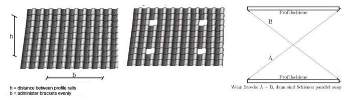
Fig. 2: Measuring of roof area
