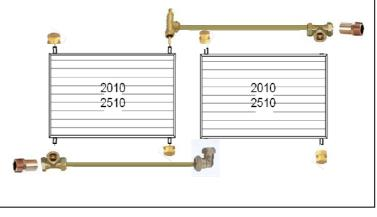
Fig. 12: Connection of collectors, vertical
