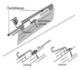
Fig. 5: Fixation of brackets
