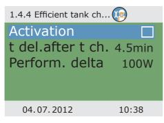
>Efficient tank charge< is activated and configured here. The solar circuit pump is controlled according to the entered heat quantity. In order to use this functionality, a heat quantity counter must be configured in the solar circuit (=> >1.1.4 Heat quantities< menu).
