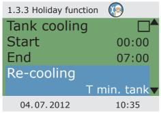
If tank cooling is activated, an appropriate time frame must be defined - this makes sense during the cooler hours of the night - by allowing the controller to dissipate as much energy as possible via the collectors.
