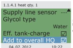
>Add to overall HQ< adds each heat quantity to the overall counter.
