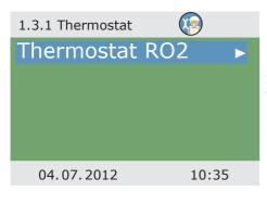
If outputs on the controller are not assigned, these channels can be used as thermostats.
