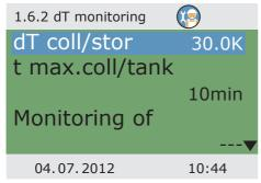
>dT monitoring< is used to define the criteria which lead to fault detection.
