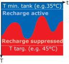
A flexible minimum temperature is thus calculated once per day which disables the recharge by the boiler.
