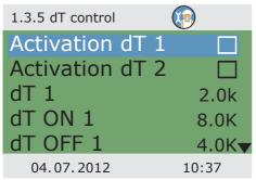
If control algorithms have been defined as >dT< under >1.3.7 Output parameter<, the appropriate outputs can be configured here.
