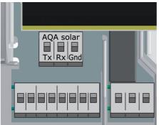
For connection, the terminals >Tx<, >Rx< and >Gnd< above the interface terminals TS1 to TS4 are provided on the extension modules.
