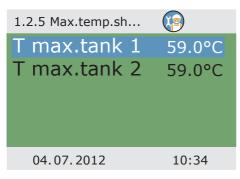
Maximum temperature of the tanks 1 and 2, to avoid excessively hot water in the tank; the tank in question is only charged to its >T max<.
