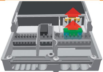
To remove the device fuse, open the terminal cover.
