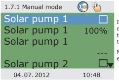
In manual mode, the individual outputs can be activated for testing purposes, e. g. to check that a pump is working properly.
