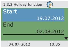
To avoid overheating of the plant, the controller will suppress yield optimization while the holiday function is activated.
