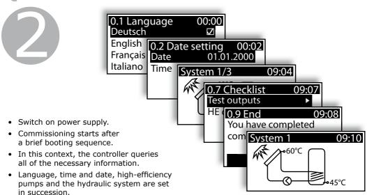
Easy operation of the controller by means of rotary encoder / OK button and esc button.
