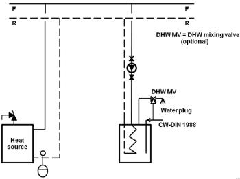
Illustration 3 (Schematic drawing- example hydraulic system heating)
